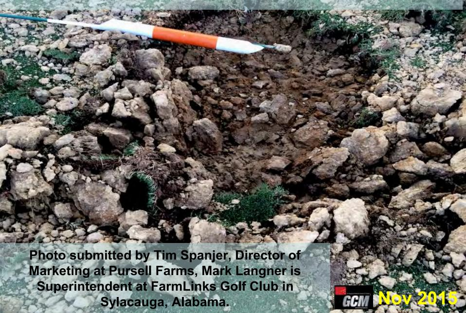
Blew 120 foot long trench 2-3 feet deep and 6-8 inches wide along irrigation pipe & blew out control boxes 300 yds away
